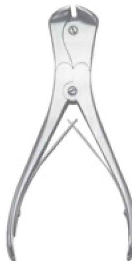
Pin Cutter SI-1401 22 cm TC for soft wire up to D = 3.5mm for hard wire up to D = 2.5mm
